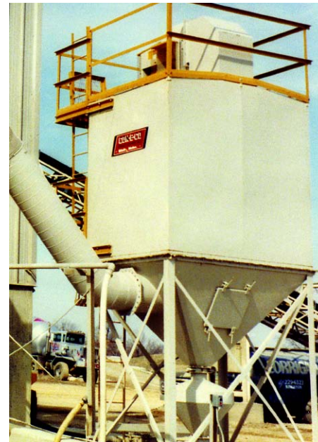
Ground-mounted dust control with automatic reclaim
