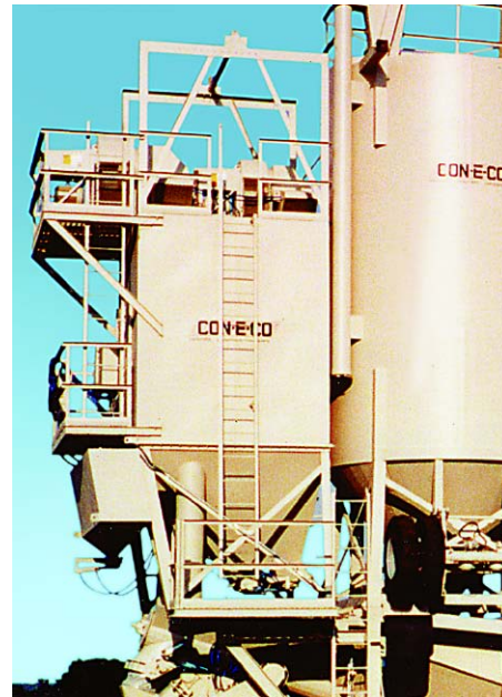
Silo and truck charging dust control with optional water holding or weighted water lifting bale and reclaim-to-cement batcher
