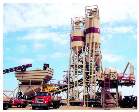
100 cubic yard, 3-compartment aggregate storage bin, 54" wide mixer charging conveyor, 475 BBL cement I storage silo, 335 BBL cement II storage silo, 12 cubic yard tilt mixer. Aggregate material handling system includes two plant-supported conveyors.
