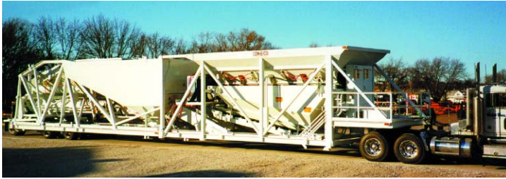
Mobile tow-away self-erecting batch plant.
